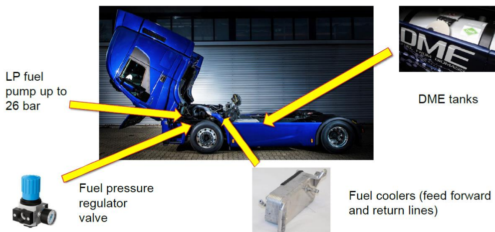
Figure 31: Necessary vehicle modifications based on standard diesel version (Daniel Klein, 2022)
