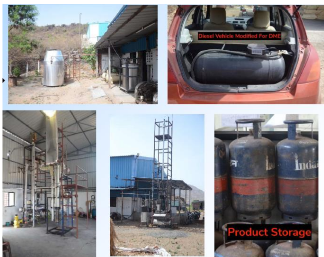
Figure 34: Pilot plant near Pune (India) demonstrating DME manufacture & use (Apte, 2022)
