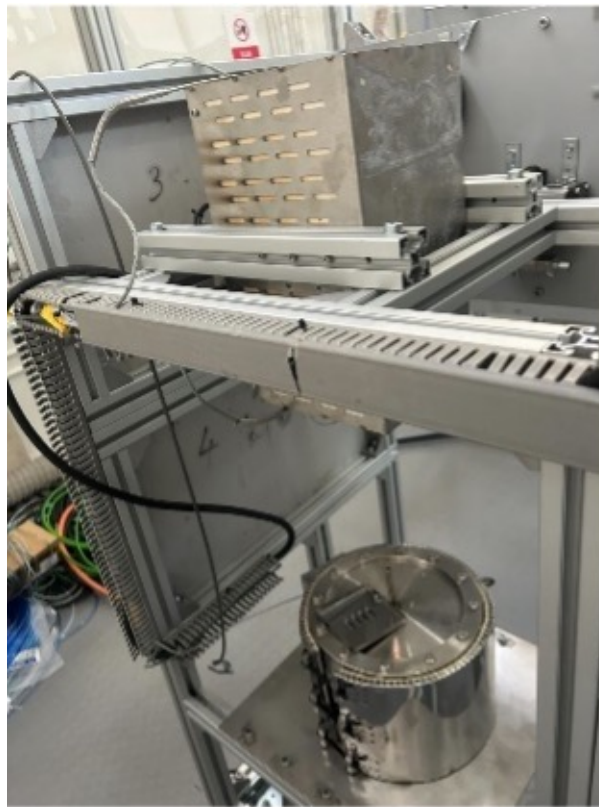
Figure 2 - overall plant view (left); H 2 , CO 2 and mixed gas heat exchangers (top right); reactor and resistance heater (bottom right)
